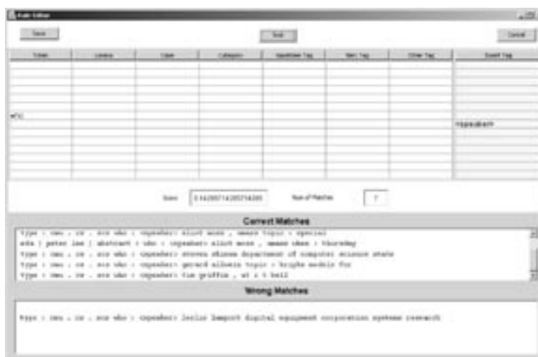
Figure 8: The Rule Editor allows to modify rules. It provides menus of possible fillers for the different fields, information on matches (correct and wrong) of the rule under development
